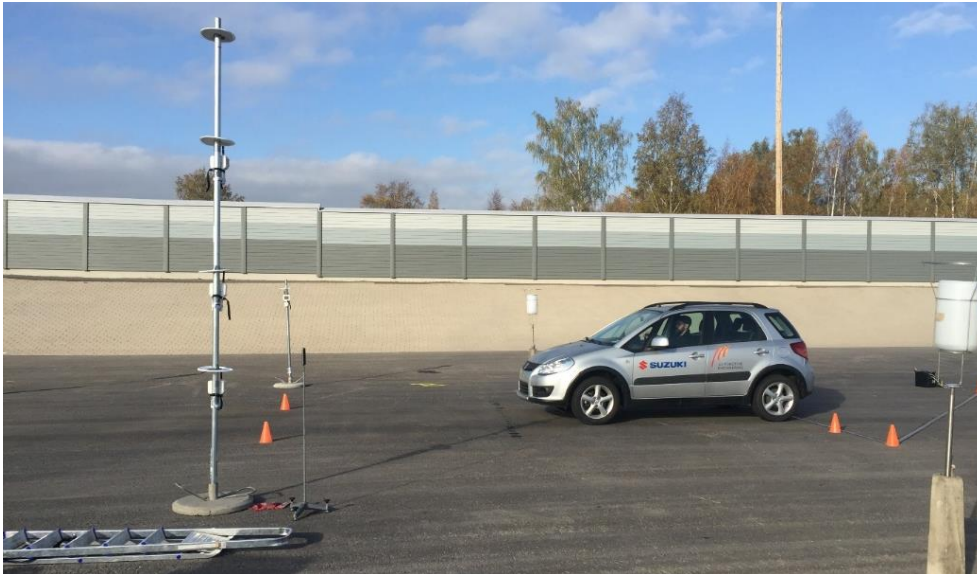
Figure 13. Measurement setup at site 1, driving O-track, passing the measurement setup where the road was straight.
