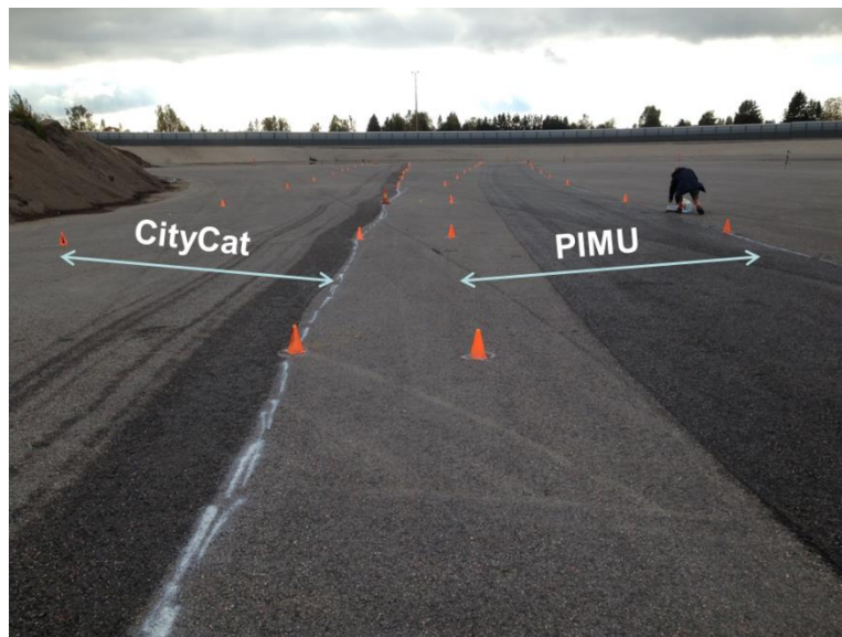
Figure 18. Wet marks on I-tracks after the cleaning.
