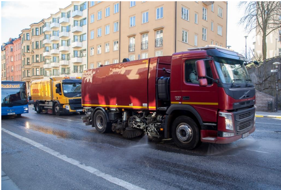
Figure 23. Flushing machine followed by a vacuum sweeper on Hornsgatan, 6th of April 2017.
