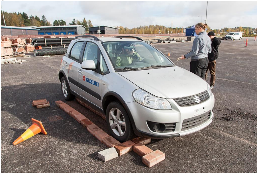
Figure 16. Brick-enclosed area for crushing test.
