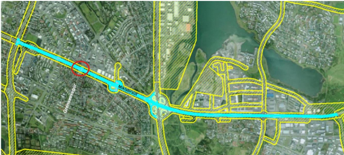
Figure 31. Road stretches for which 24-hour average of salting amount is given. Blue stretch area, A = 171\,950\text{ m}^2 ; blue stretch length, L = 5640\text{ m} ; blue stretch average width of roadway, w = 30.5\text{ m} ; lane width 3.75\text{ m} ; average number of lanes on blue stretch 8.1 . Data and image from the Road Administration upon request.
