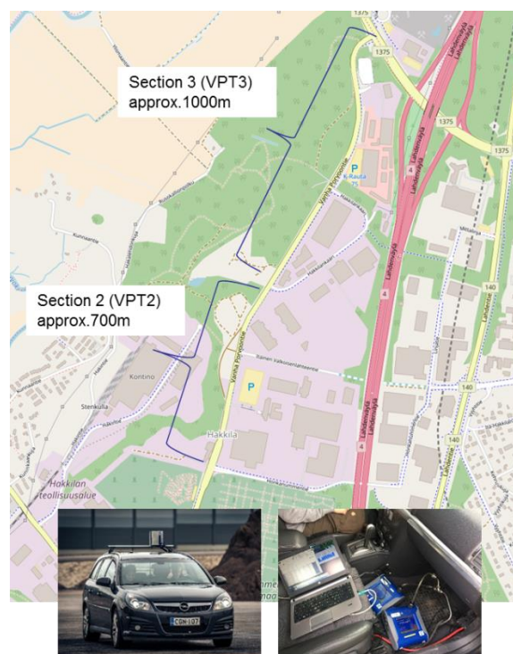
Figure 1. Vanha Porvoontie segment used for the on-road measurements of tyres with the Vectra vehicles
