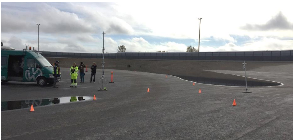
Figure 15. Measurement setup at site 3, driving O-track, passing the measurement setup where the road was curved. At this site the Sniffer, measuring PM10 with a TEOM, was standing at the same place as the measurement setup
