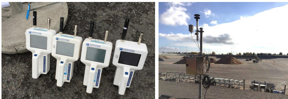
Figure 11. The Lighthouse instruments used for measuring PM10 during the Vantaa campaign (left) and meteorology station (right).
